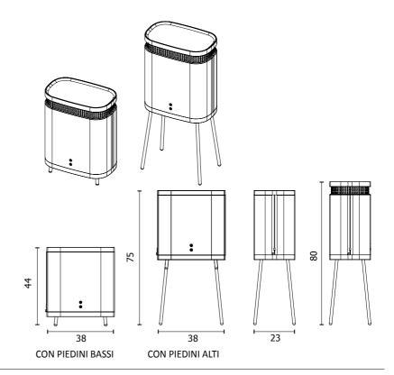
DUE SET DI PIEDINI CON ALTEZZE DIVERSE FORNITI DI SERIE.
