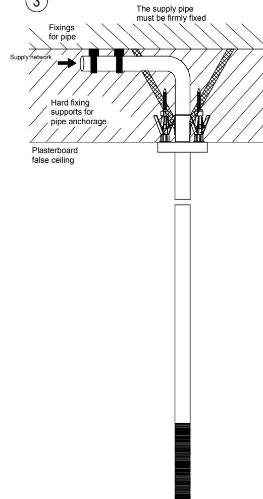
ATTENTION: In the second and third case hard fixing supports are not provided in the box but they need to be realized by the installer during the installation phase
